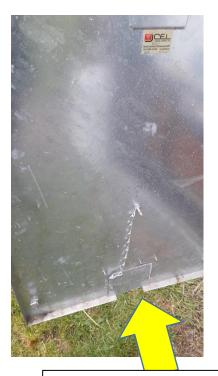
Hatch is opened by unscrewing bolts by hand on the back and hanging on the pin.
